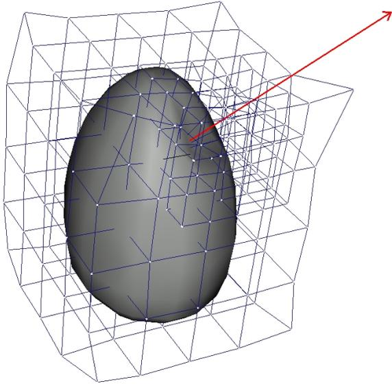
**Figure 1:** The finite mesh and the data can have different resolutions in addition to the adaptive level of detail for finite mesh.
