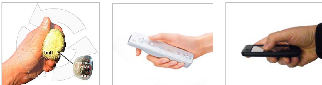
Figure 5: Wireless mid-air devices for interaction with presentation technologies – (a) SOAP [4], (b) Wii remote [16] and (c) iPhone [18]. These devices have the advantage of being inexpensive, simple and intuitive to use, offering access to additional controls and user mobility.
