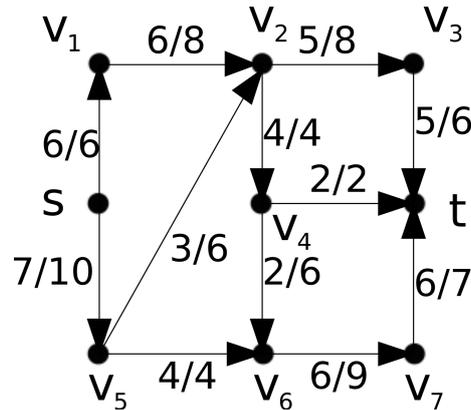
Figure 2: The network  $(G, c, s, t)$ . The tuples at the edges have the form (flow/ capacity).
