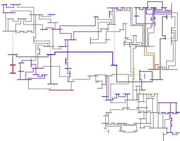
Figure 6: Per-unit voltage mapped to discrete colors of bars. Blue  $\leq 0.96$  and Red  $\geq 1.04$
