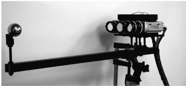
**Figure 3:** The single lens setup with an RGB beamsplitter (left), and the simpler setup with three separate lenses and RGB color filters pointing at a reflective sphere (right). Both use three separate, unmodified but reprogrammed C55 camera units.
