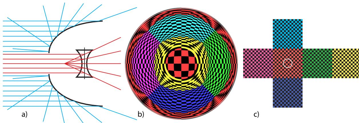
Figure 1: **a)** A principal sketch of the mirror and lens setup, with reflected and refracted rays for the parallel projection case. **b)** An image of a checkered environment map, as displayed in **c)**, as projected by the setup. The field of view of the central lens is about  $30^\circ$ , represented by the white circle in the cube map.
