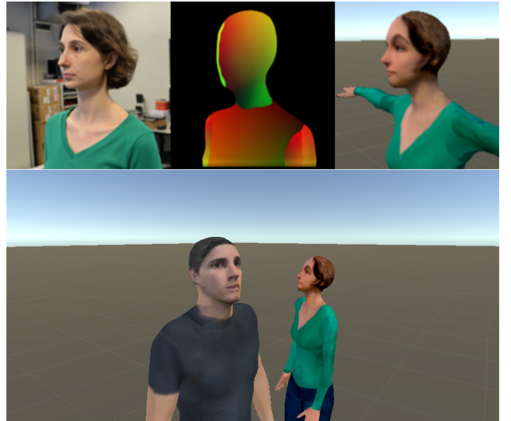
Figura 1: 3D reconstructed models. Here we apply the texture captured in the first step over the mesh generated by the second.
